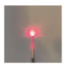
CORONA Infinite Ring Fiber® delivers a homogenous radial pattern along a continuous ~4mm section, without front firing.
